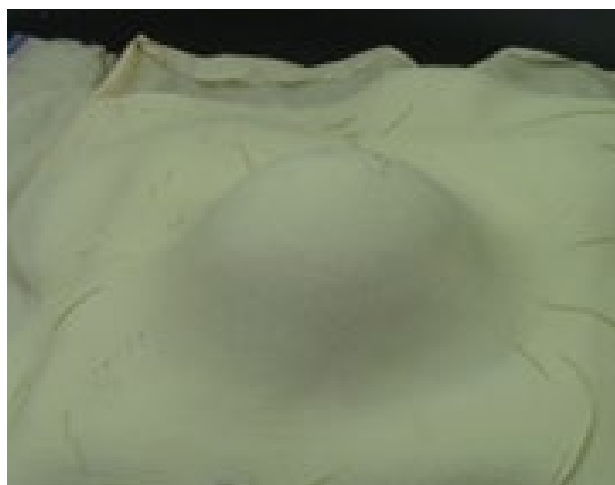
10 11 12 13 14 15 16 17 18 19 20 Fig. 14. Hemisphere covered by mesh layer jamming sheets (16 sheets). The 21 laminated sheets followed the sphere without wrinkling and maintained their 22 shape by discharging the internal air.
