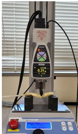
Fig. 16. A three-point bending flexural test in which a layer jamming element placed on supporting pins with a spacing of 64 mm was pressed down at a speed of 50 mm/min using an indenter whose cross-section has a semicircle with a radius of 6 mm.
