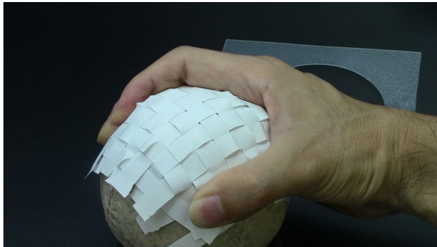
Fig. 3. A view of wrapping a ball of 97 mm diameter with a woven structure of paper strips (width = 10 mm). A woven structure of paper strips fits a curved surface; however, it lifts off the surface when the radius of curvature is small, resulting in gaps.
